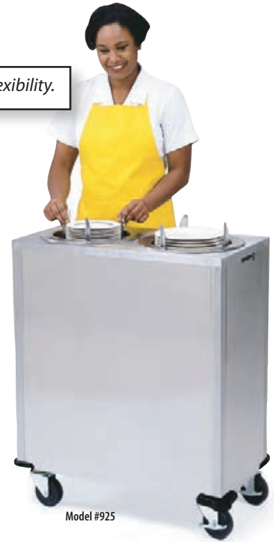
1. Height Adjustment – Simply detach or attach springs to adjust tension for the height level you desire. 2. & 3. Adjust-a-Fit® Size Adjustment – Easily re-position and lock the dish guides with a turn of the wrist. No tools necessary!
