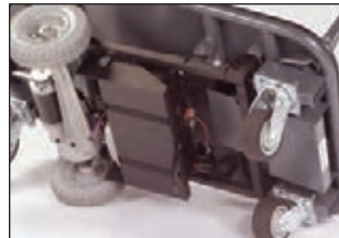
Sealed AGM maintenance free batteries.
